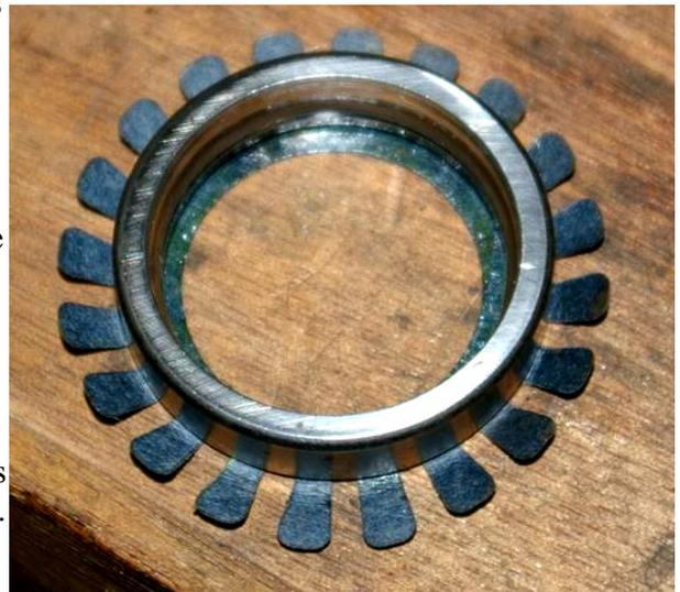
such as Evo-Stik. If the insulator has one shiny side, it should be outermost, i.e. the non-glued side.
